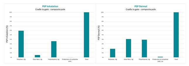
Figure 5: ProScale result for inhalation (left) and dermal (right) for the composite utility pole.
