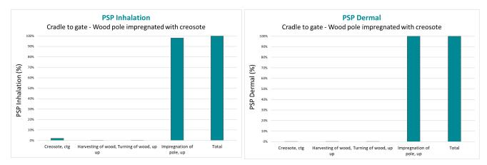
Figure 4: ProScale result for inhalation (left) and dermal (right) for the wood utility pole impregnated with creosote.
