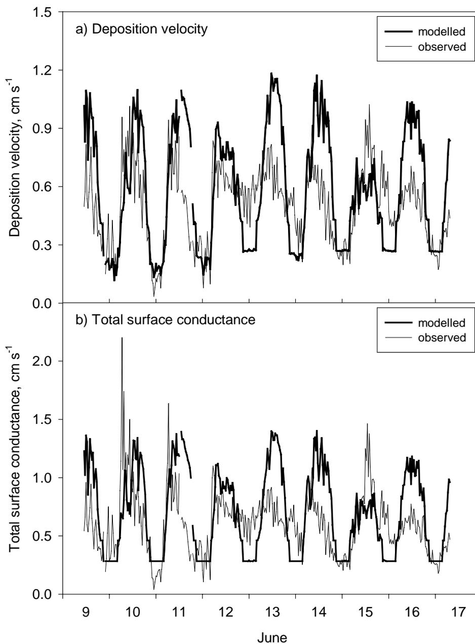
**Figure 13.** Observed and modelled dry deposition velocities at 21 m (a) and total surface conductances (b) from 9 to 17 June 1994 in a Norway spruce forest at Ulborg, Denmark.
